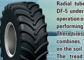
Radial tubeless tires 800/70R32 DF-5 and 680/85R32 DF-5 under the brand VOLTYRE-AGRO are designed for operation on combines of Russian and foreign production, performing work in agriculture.
